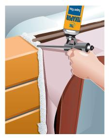
TEKAPUR PU - foam Super Flex is gun grade one-component polyurethane foam with very high elasticity used for fixing and mounting. It hardens with air humidity.
