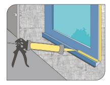
**Tekadom Acryflex** is a one-component extremly flexible plastoelastic sealant based on special acrylic dispersion.
